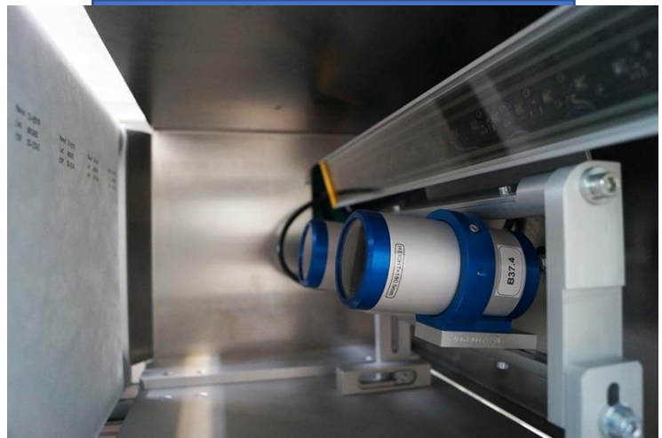
Harletray multifunctional camera for OCV/OCR control
